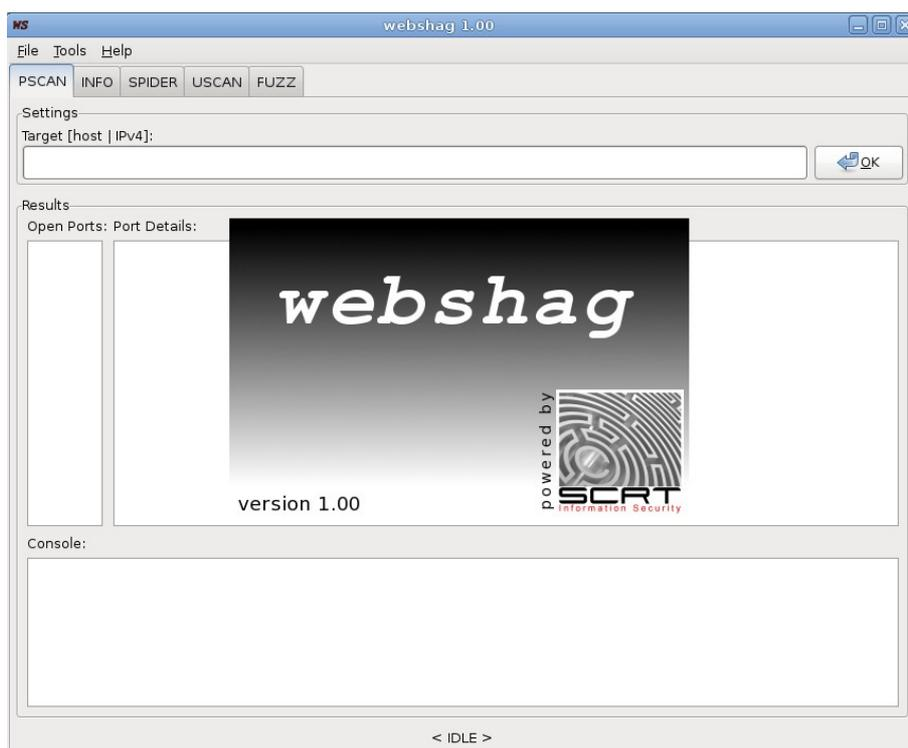
To switch between the audit module, use the tabs located below the menu bar. Note that execution of modules is multi-threaded, it is thus possible to run several modules at the same time. The status of each module is indicated on bottom: <IDLE> or <RUNNING>.
